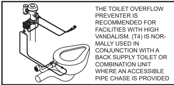
(T4)- MANUAL RESET TOP FOUR OVERFLOW PREVENTER (REQUIRES (FV) HYDRAULIC FLUSH VALVE AND ACCESSIBLE CHASE)
