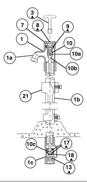
\*These parts are accessible from face of hydrant by removing face nut.
