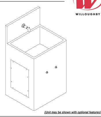
To specify fixture and accessories, use the Model Number and Options page. Example: To specify a Front Mounted Service Sink, 22" x 20" with plain end spout, dual temp. pneumatic metering valve ligature-resistant pneumatic push buttons, and removable 'p'-trap Use the following Willoughby Model Number: SS-2220-FM-FA-SE-PML2-PBH-RPT
